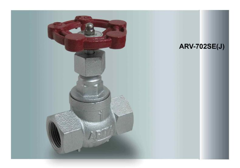
The body and bonnet of globe valves are casted from ductile iron. This provides the valves with superior physical and chemical properties over cast iron in tensile strength, shock, vibration, and corrosion. The stainless steel stem with trapezoidal thread allows it to withstand higher load and longer service life. The seat and disc are made of stainless steel with fine finished surfaces and they are self aligned to give a long leak free service.
